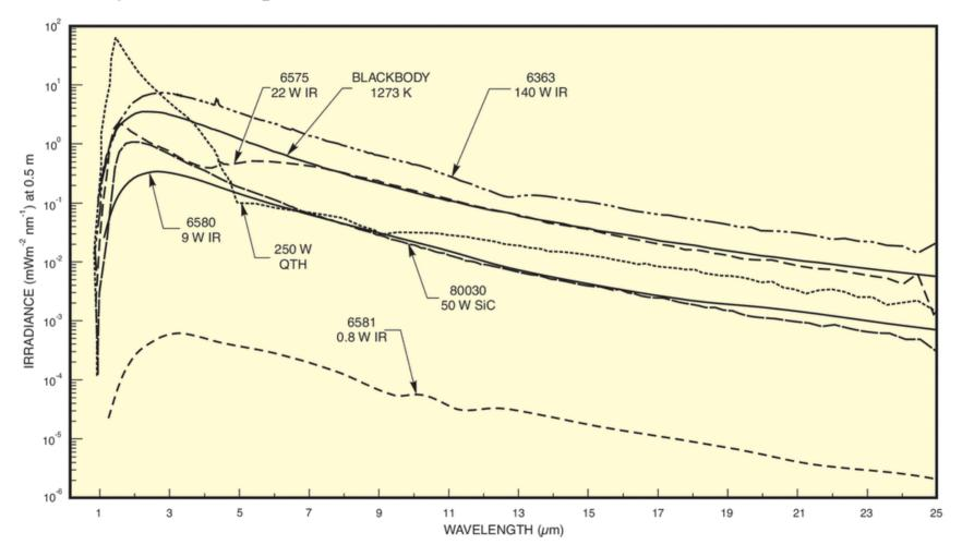
Sources: SiC – glowbar, QTH – quartz halogen, 6580 and 6581 are Oriel IR sources (inexpensive), 6575, 6363 - different design (hotter)
