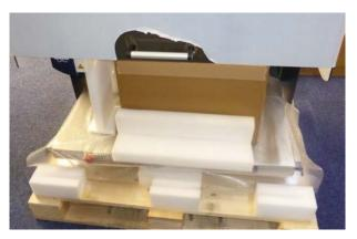
Figure 4.10: Protect front shield with a spacer foam
