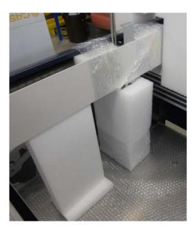
Figure 4.1: Placing Foam Parts to protect Z-module & Y-Arm
