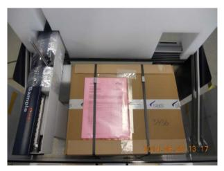
Figure 4.11: Place and fix the accessory box on the deck
