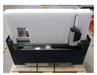
Figure 4.6: Stabilizing the arms and the X-rail with a foam block
