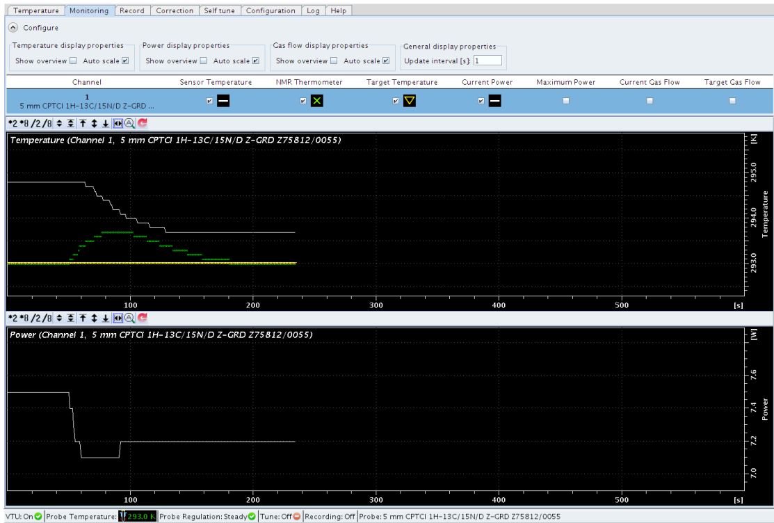
Figure 4.12: Monitoring of the sensor and the sample temperature in edte during a TOCSY experiment
