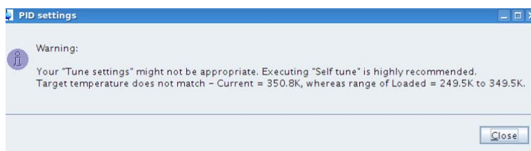
Figure 5.14 Warning message if there are no valid PID parameters for the desired temperature.
