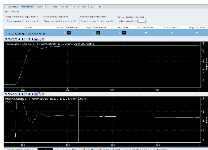
Figure 5.22 Example of a temperature jump of 80 K, the sensor temperature is depicted on the top, the heater power on the bottom.
