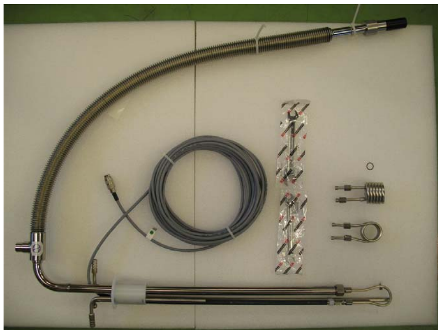
Figure 4.12 Heat exchanger kit with Johnston coupling and different inserts
