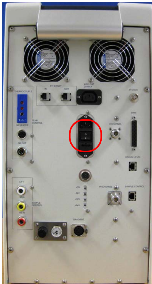
Figure 3.1 Location of the Console Emergency Shutoff
