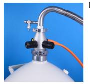
[24] Then attach the cap on the NITROGEN GAS OUT port (red)
