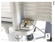
[12] Adjust the two brass elements (1) on the support plate with an Allen key to fix the position of the probe. Leave a ~1-2 mm gap between the probe and the brass elements. This step only needs to be performed once during the first installation of the Cryo-Probe Prodigy.
