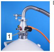
[23] First attach the cap on the LIQUID NITROGEN IN port (blue)
