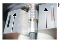
[4] Press the MTM against the bottom of the CryoProbe.
