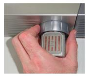
[6] Support the Exhaust Heater/Vacuum Operator with the palm and grab the mounting ring (1).
