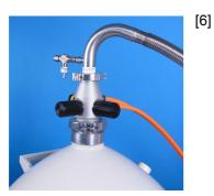
6] Then attach the cap on the NITROGEN GAS OUT port (red)
