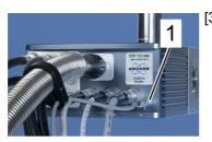
[3] Connect the Transferline ID cable (1) to the front of the CryoProbe.
