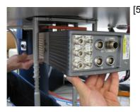
[5] Align the tube of the CryoProbe with the shim system. With the help of a second person, carefully insert the CryoProbe all the way into the shim system, allowing the probe body to be guided by the rear guiding rails. The CryoProbe should enter the magnet bore straight and without any resistance.
