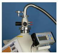
[3] Connect the display connection cable and the power supply of the scale to the display unit.
