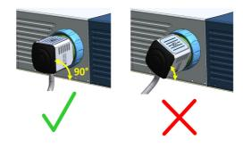
Figure 6.12: Mounted Exhaust Heater.
