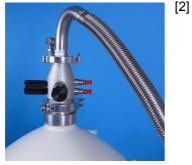
Remove the black port caps from NITROGEN GAS OUT port (red) and LIQUID NITROGEN IN port (blue).
