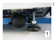
[1] Lower the three fixation stands (1) under the Prodigy Unit to prevent it from rolling off.
