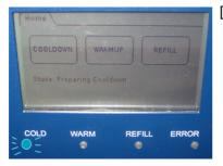
[4] After pressing <COOLDOWN> the displayed status changes to "State: Preparing cooldown" and the blue LED starts flashing Figure 7.3.
