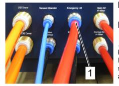
Figure 5.12 Emergency lift connection
