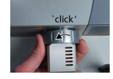
Figure 6.18: Pulling the mounting ring.
