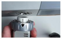
Figure 6.19: Mounting ring can be released. Pulling out the Exhaust Heater/vacuum Operator.
