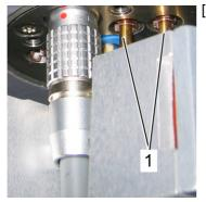
[3] Align the adaptor's bolts (the longer pins (2) in Figure 6.23) into their counterparts on the bottom of the CryoProbe Prodigy (Figure 4).
