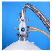
[4] Plug in the orange 10mm twin gas tube. Connect the other end to the Prodigy Unit according to "LN2 Dewar" on page 53.
