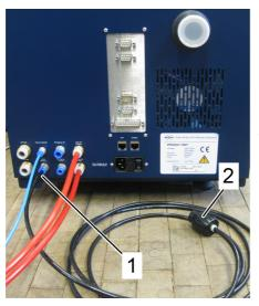
Figure 5.9 Active warmup plug connection.
