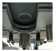
Figure 6.20: Connector on the CryoProbe.
