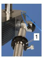
Figure 6.15: Attached vacuum hose.
