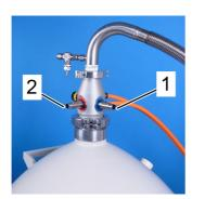
[6] Remove the black port caps from LIQUID NITRO-GEN IN port (blue) (1) and NITROGEN GAS OUT port (red) (2) of the LN2 Dewar Adaptor by turning it counter-clockwise.
