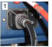
Figure 5.19 Power supply connector
