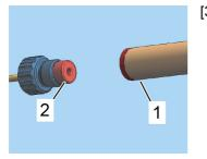
[3] Screw the extension on the dewar end connector of the Transferline.
