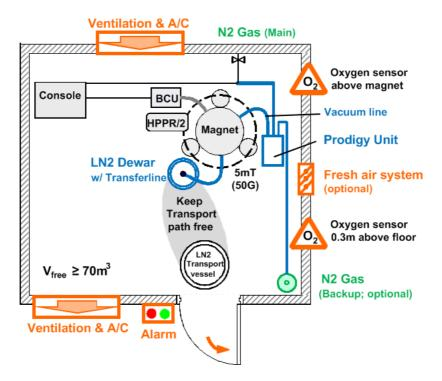
Figure 2.2 Example for a CryoProbe Prodigy Installation
