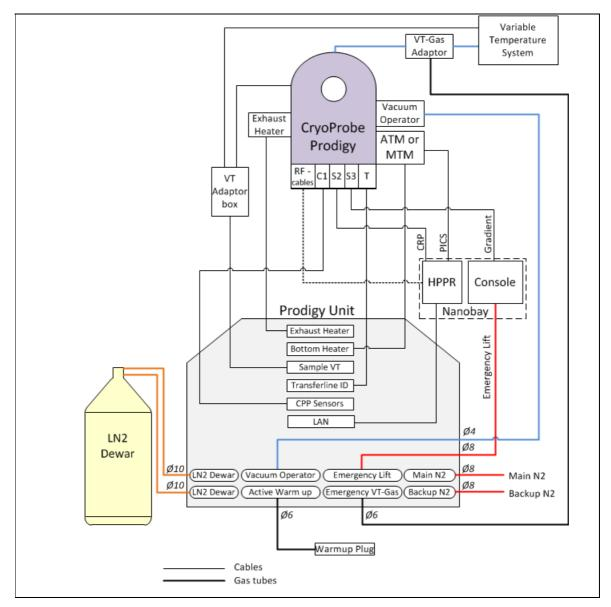
Figure 5.5 Cable and gas tube connections of the Prodigy System.
