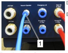
Figure 5.8 Vacuum Operator connection
