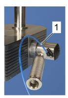
[3] Connect the 4 mm blue gas tube to the Vacuum Operator (1)
