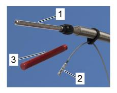
CryoProbe-side end (1) of the Transferline with Transferline ID cable (2) and red Transferline-cap (3).
