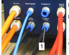
Figure 5.11 Emergency VT gas connection
