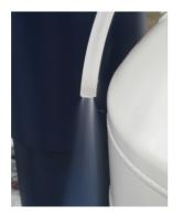
[19] Stop the nitrogen flow immediately, when LN2 overflows and spills out through the overflow hose (Figure 4.12) or the scale indicates a weight difference of ~80 kg for a 100 L LN2 Dewar.
