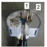
To install the MTM the slot of the MTM has to be centred around the VT adaptor (1) as shown in Figure 6.23. Please note that the VT adaptor and the sample heater cable are already connected to the bottom of the CryoProbe at this stage (Figure 6.24).
