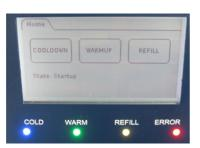
Figure 7.1: Prodigy Unit display and LEDs during startup.
