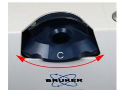
Select the desired position of the rotary disk by rotating it until it locks in place. You will hear an audible click.
