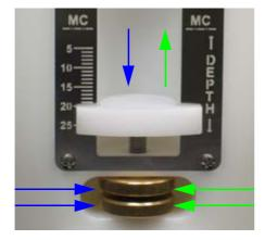
Figure 7.5 Adjusting the Sample Depth
