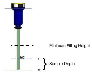
Figure 7.2 Example: Sample Tube with Sample Depth 20 mm
