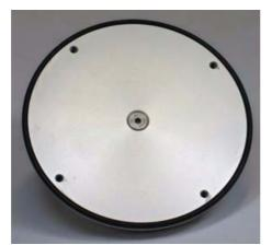
6. When you rebuild the unit do not forget to replace the O-Ring seal.
