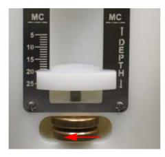
Figure 7.4 Loosening the Knurled Screws
