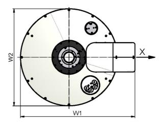
Figure A.2: Dimensions of the cryostat (top view)
