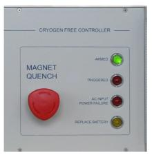
Figure 5.15: Emergency button MAGNET QUENCH on the BCFC front panel
