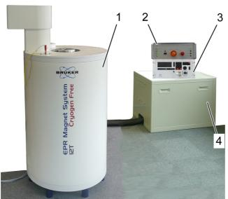
(1) EPR 12T Cryogen Free Magnet System
