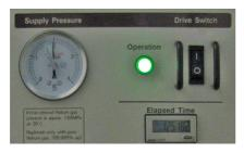
Start the compressor CNA-61 using the "DRIVE SWITCH".
