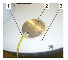
Figure 5.7: Mounting the earthing cable
