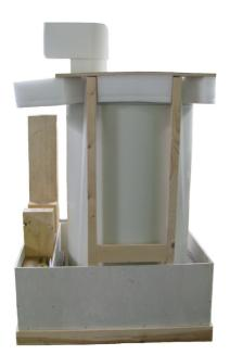
The magnet system is packed in a transport box. It is secured inside with tightening straps against tilting and moving.
