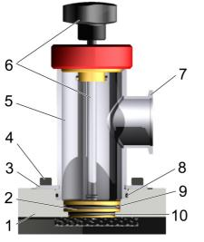
3. Install the valve stem (6) onto the sealing plug (2) and tighten it slightly. Do not yet fix the valve operator body (5) to the cryostat.
