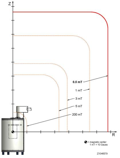
Figure A.3: Fringe field plot of the EPR 12T magnet system Scale division is 0.5 m.
