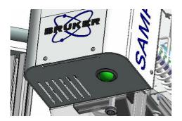
Before carrying out any manipulation, look up to the Sample Mail housing and check that the control lamp is lit up green. This means that there are no more samples in the magnet and that the system is ready to accept a new sample.
