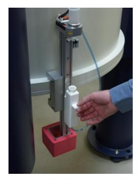
Take hold of the slider and pull it down to the stop.
