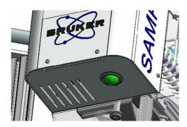
The sample travels back into the loading compartment, and the status control lamp then switches to green again. The sample can now be removed.
