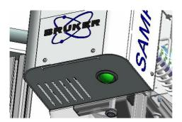
Before any manipulation is done, look up to the Sample Mail housing and check that the control lamp is lit up green. This means that there are no more samples in the magnet and that the system is ready to accept a new sample.
