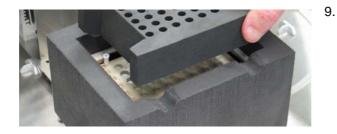
. Cover the cooling rack with the cap.
