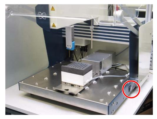
The robot ON/OFF switch is located on the right side of the deck tray:
