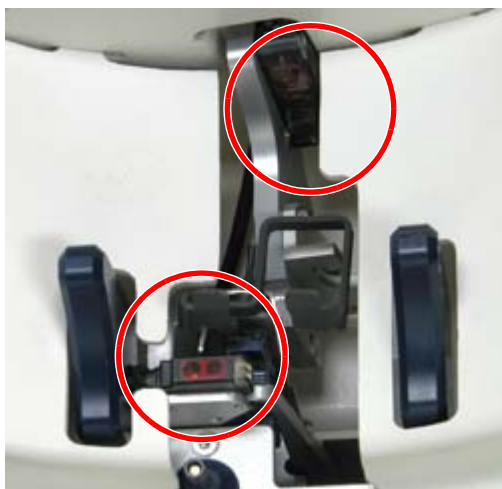
Figure 9.3 Carousel Light Barrier
