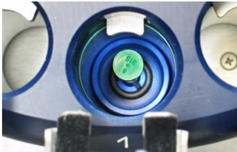
Figure 10.1 Sample Stuck in the Carousel
