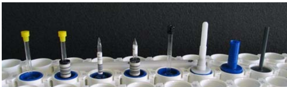
Figure 4.2 Example of Samples That Can be Used with SampleXpress Lite
