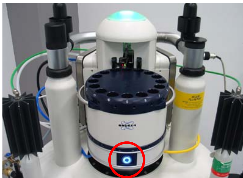
Figure 8.1 Location of the Power Button
