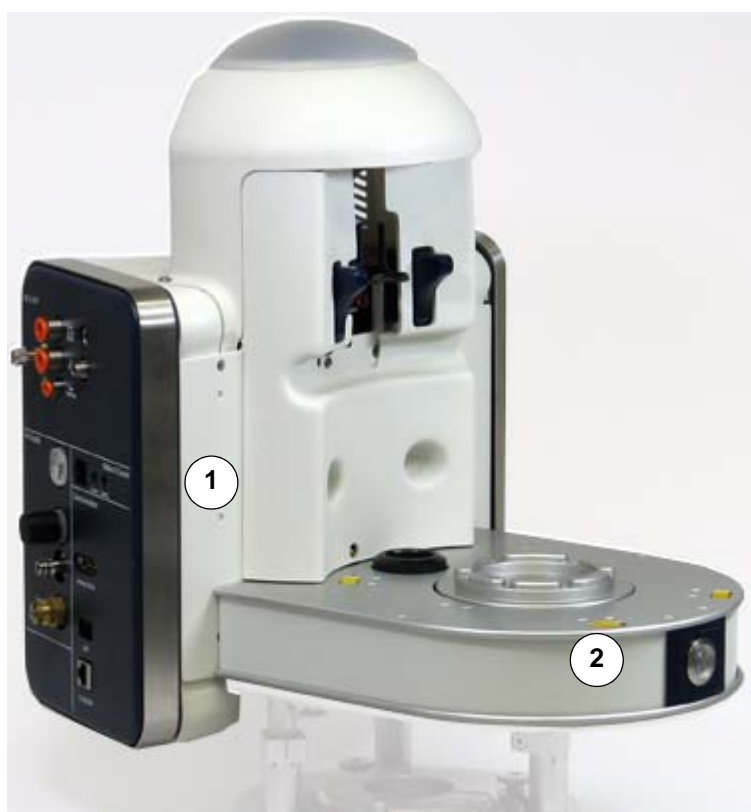
Figure 5.3 Base Unit and Carousel Base Mounted on Base Plate
