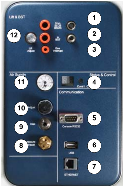
Figure 5.7 Connections Left Side
