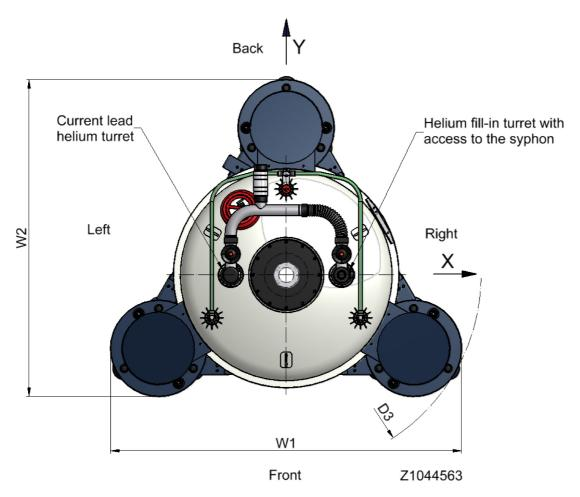
Figure A.2: Dimension Cryostat - Top View
