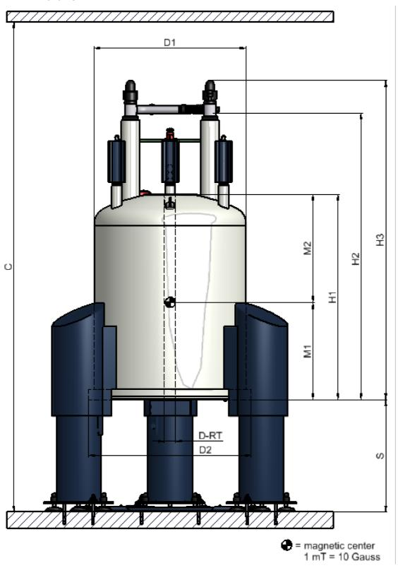
Figure A.1: Dimension Cryostat - Front View
