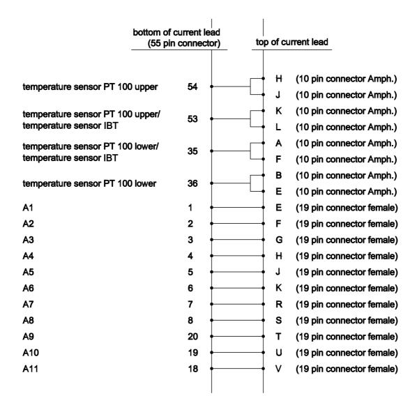
Figure A.11: Wiring Diagram Magnet - Diagnostic and Temperature Sensors
