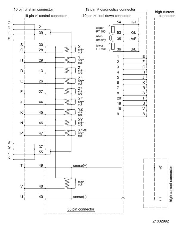
Figure A.9: Wiring Diagram Magnet
