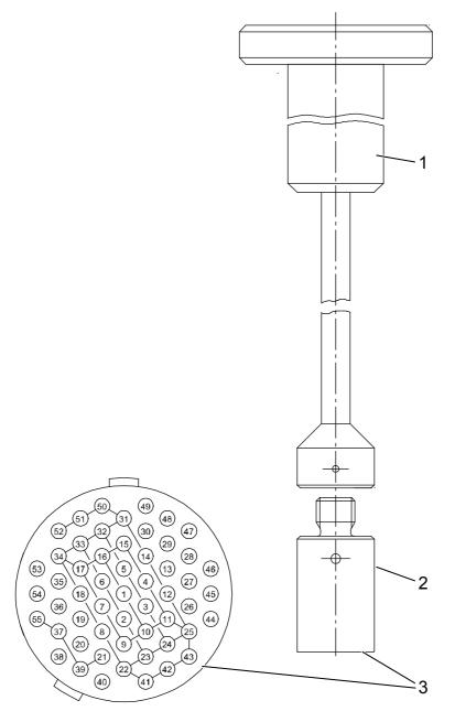
Figure A.12: Shorting Plug 55 pins
