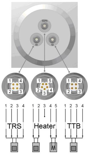
Figure A.7: Wiring Diagramm Temperature Sensors
