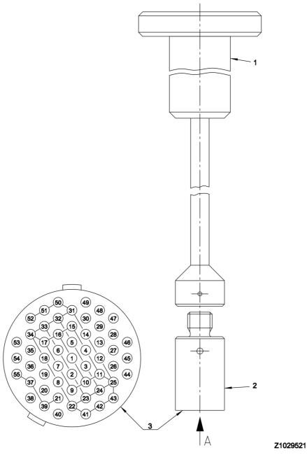
Figure A.12: Shorting Plug 55 pins
