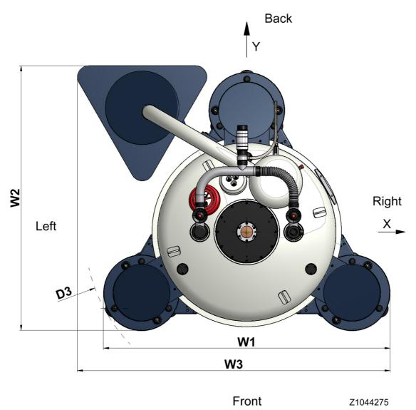
Figure A.2: Dimension Cryostat - Top View
