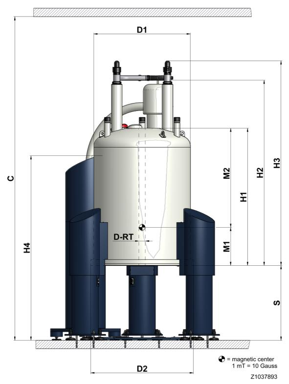
Figure A.1: Dimension Cryostat - Front View
