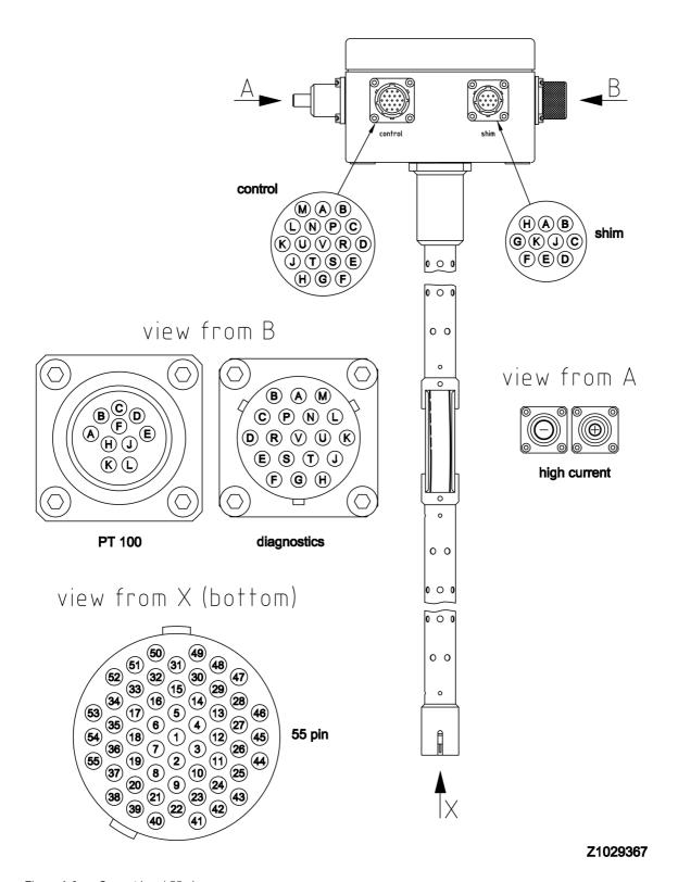
Figure A.8: Current Lead 55 pins
