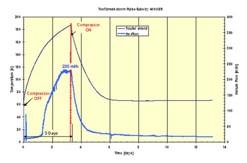
Figure 6.2: Temperature profile during Cryogenic Refrigerator failure
