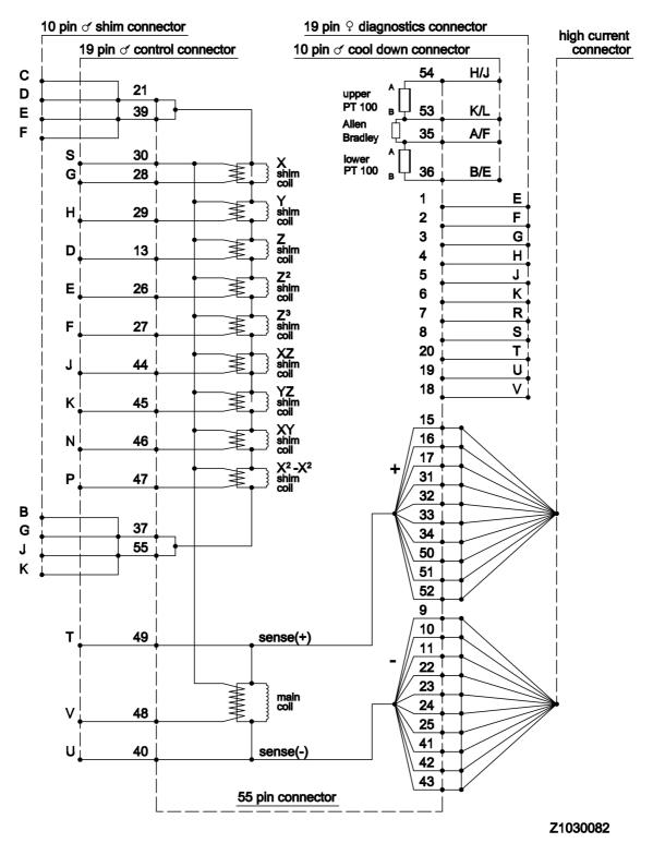
Figure A.9: Wiring Diagram Magnet
