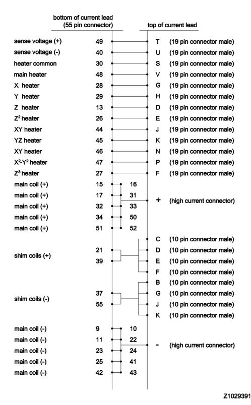
Figure A.10: Wiring Diagram Magnet - Control
