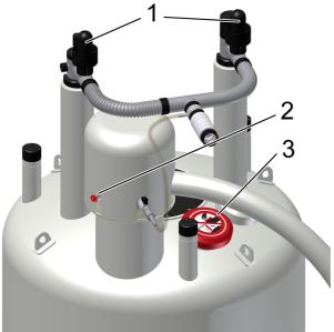
Safety Devices of the Cryostat
