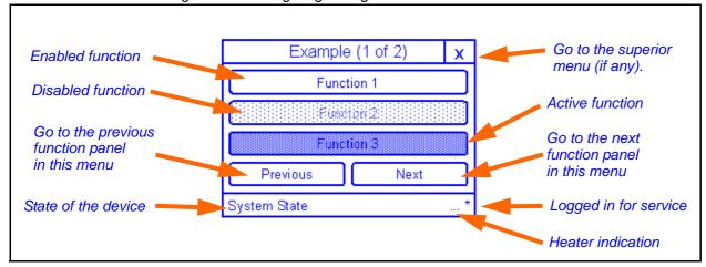
It is possible to protect the "service" menu by setting a code in "User Settings" on the web interface. If no password is set you do not have to log in and out. The "Logout" button is then disabled.
