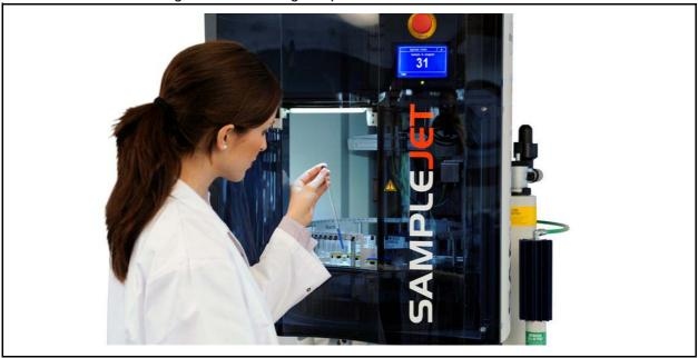
To access a sample in the openshop ring storage use the "Load Sample" function in the "Main menu" of the SAMPLEJET display. This will rotate the chosen sample position to the front door.
