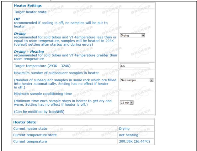
Figure 13.5. Heater windows on the display
