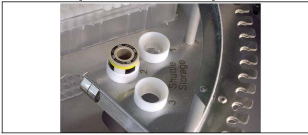
Take care to hang the tubes correctly into their holders. The caps are guided by the holder and in most cases the caps will fall into the right position when inserting the tubes. If a tube is not hanging correctly, the gripper will try two times to grab the cap because the first attempt to grab will often push the cap down in the holder. The second attemp has then no problem to grab the cap correctly.
