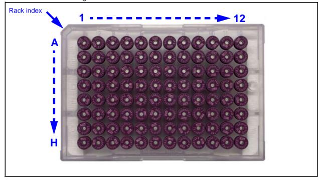
Figure 5.21. The enumeration of the rack
