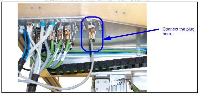
Figure 14.2. Where to connect the REMOTE CONTROL
