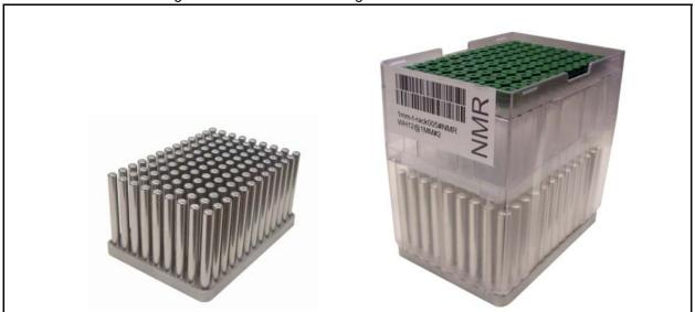
Since the heat exchanger has a much bigger mas then the rack with the tubes, the temperature stays constant when inserting and removing racks. The rack slots do not need to be covered when not in use.
