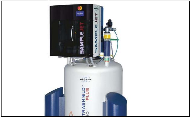
The SAMPLEJET is a push-button system, which runs under complete computer control enabling modern interfaces like Ethernet and a comprehensive communication link for service and diagnostics with web based mechanisms. It's built-in electronics control and continuously monitor all operations needed for an entirely automatic sample handling.
