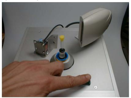
The B-BCE unit will now try to read the barcode, if the reading is successful the "Good Read" light will light up. The motor of the B-BCE will then stop and the Tube ID will be copied into the Tube ID field of the Manual Preparation window of SampleTRACK.
