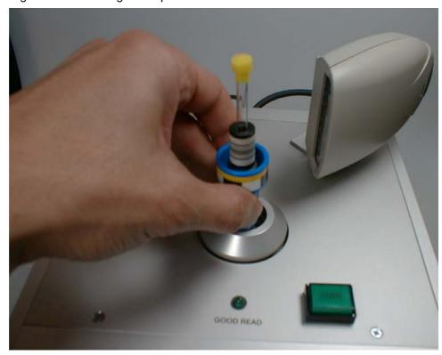
Figure 3.2. Inserting a Sample in to the B-BCE
