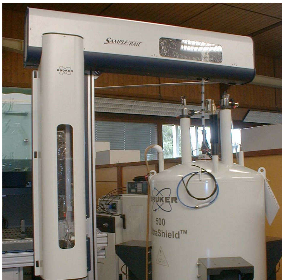
Figure 3.4. Example of a BSR VAC System
