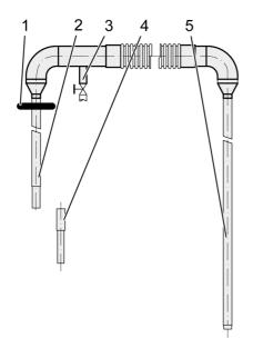
For the transfer of liquid helium a helium transfer line is necessary. The helium transfer line is vacuum-insulated and the vacuum has to be refreshed regularly using a vacuum pump at the vacuum valve (3) of the transfer line.
