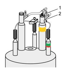
10. Remount the plug (1) to close the helium fill-in turret (2) immediately to prevent air from entering the turret.
