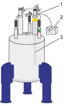
Figure 4.4: Helium Level Sensor
