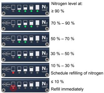
Figure 3.4: Display of the Nitrogen Level Sensor
