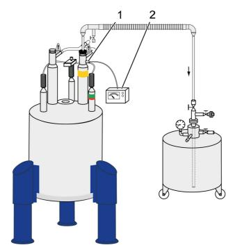
26. Switch the helium level measurement at the BSMS Service Web to continuous measurement mode ("Fill Mode").
