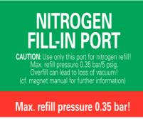
The nitrogen fill-in turret on the magnet system is marked with a green and red colored label.
