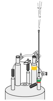
1. Remove the heat exchanger from the nitrogen fill-in turret.
