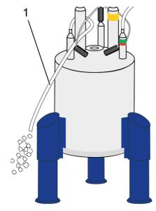
14. Check if gas is escaping from the Teflon® hose (1) at the nitrogen turret used as exhaust. This indicates that the turret is free and not blocked with ice.
