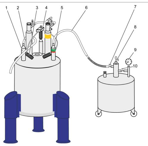
Figure 1.1: Setup of the magnet system during the nitrogen refilling procedure
