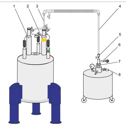
Figure 1.4: Setup of the magnet system during helium refilling procedure
