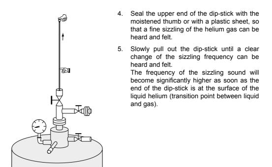
Figure 4.7: Fluid level measurement in the transportation dewar – step 2
