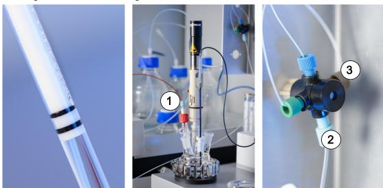
Figure 6.4: From Left to Right, Glass Flow Tube O-Rings, Vessel Connections ,and Flow Interface Valve
