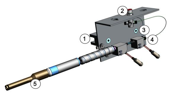
Figure 4.3: InsightMR Flow Tube Assembly, Flow Tube Protector and Flow Interface
