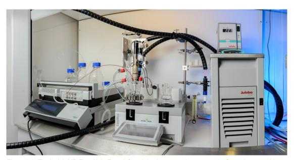
Figure 6.3: The InsightMR Flow Unit. From left to right: the pump, the reactor, the flow tube assembly secured with a clamp stand and the thermostat.
