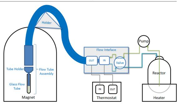
Figure 9.1: InsightMR Flow Unit Laboratory Setup
