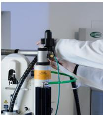
Figure 7.2: Mounting the Insulated Transfer Line
