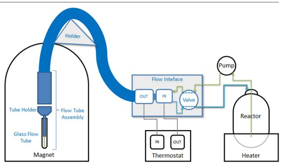
Figure 8.1: InsightMR Flow Unit Laboratory Setup
