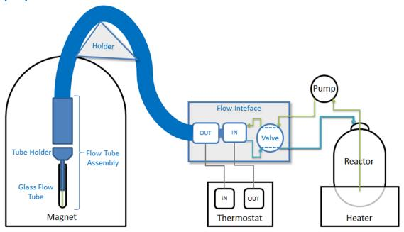
Figure 4.2: Recommended Laboratory Setup
