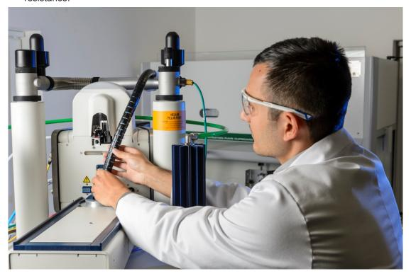
Figure 7.1: Inserting the Flow Unit Assembly into the Magnet
