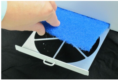
Figure 8.4: Removing and Installing the Filter
