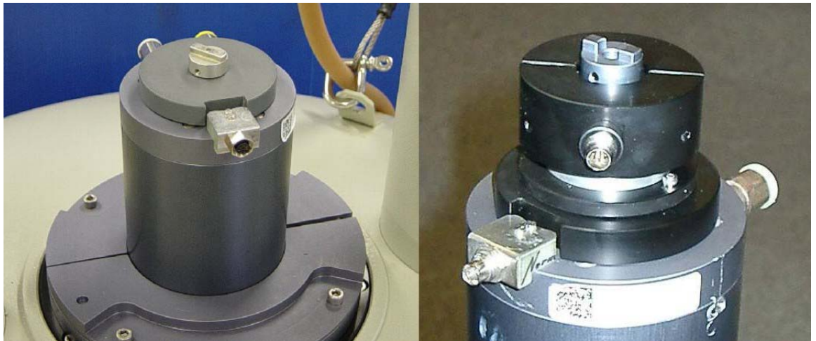
Figure 2.2: Drive Shaft in the Old Gray Style Shim System.
