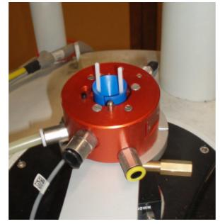
Figure 6.3: Inserting the Guide into the Shim Upper Part
