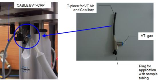
Figure 5.1: Bottom of CryoProbe (left) and T-Piece (right)
