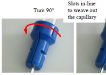
Figure 6.9: Removing the Insert Guide
