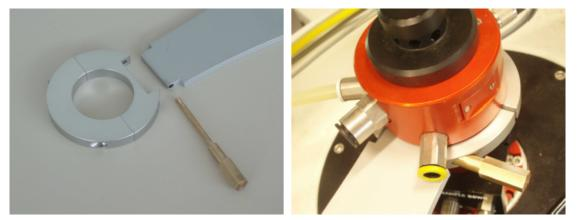
Figure 5.5: Mounting the CryoFIT Holder on the Upper Part of the Shim System
