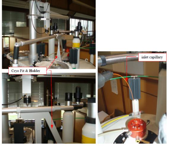
Figure 6.7: Inserting the Capillary
