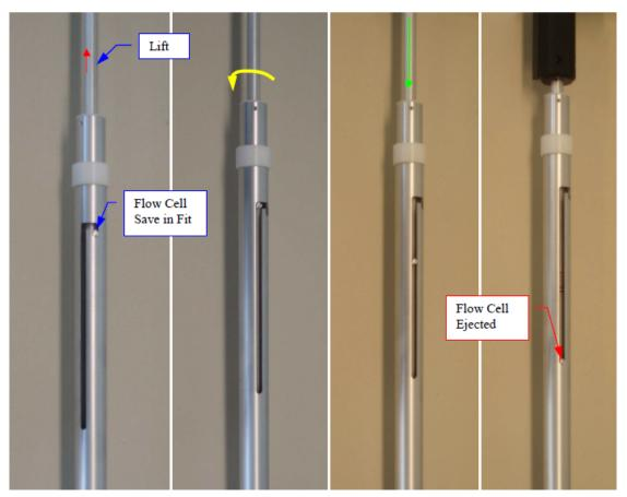
Figure 6.12: Inserting the Flow Cell
