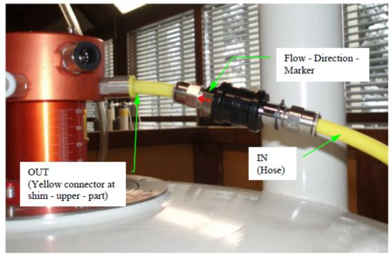
Figure 5.2: Valve Mounting
