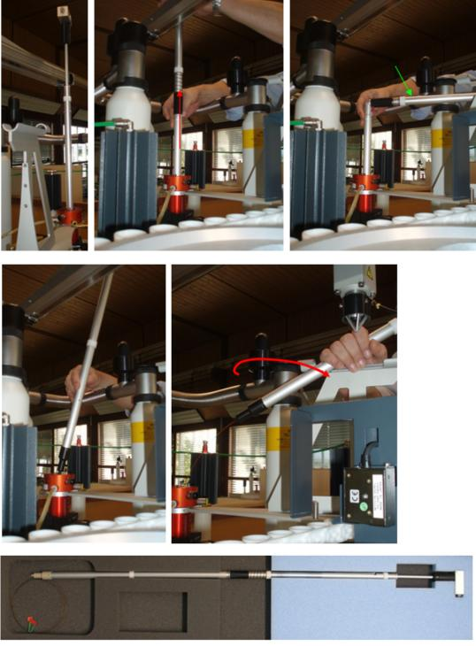
Figure 7.3: Removing the CryoFIT
