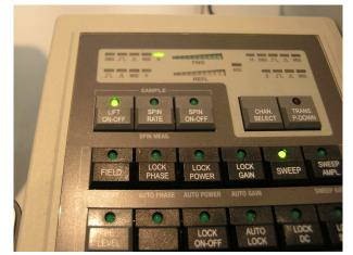
Activate the sample lift so that the insert guide is lifted:
