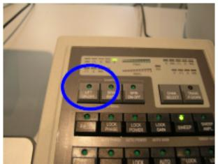
Figure 6.10: Switching Off the Sample Lift
