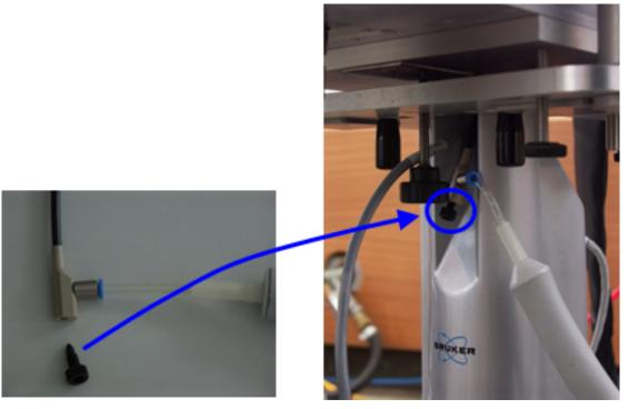
Figure 7.4: Plugging in the T-Piece
