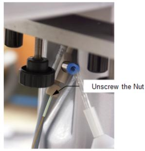
Figure 7.1: T-piece and Disconnected Outlet Capillary
