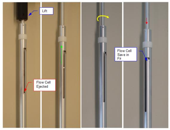
Figure 7.2: Removing the Flow Cell
