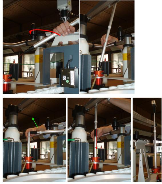
Figure 6.11: Inserting the CryoFIT
