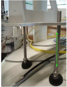
• Adjust the length of the bracing holder on the magnet until the plate is horizontal.
