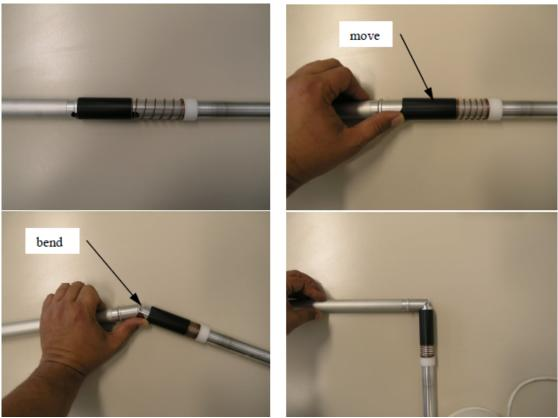
Figure 6.6: Bending the Frame Joint
