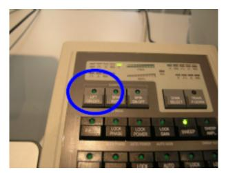
Figure 6.4: Switching Off the Sample Lift
