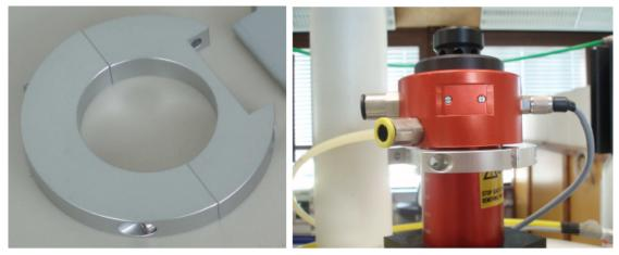
Figure 5.3: Bracket Mounting on the Shim Upper Part
