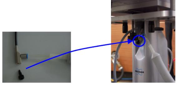
Figure 6.5: Unplugging the T-Piece
