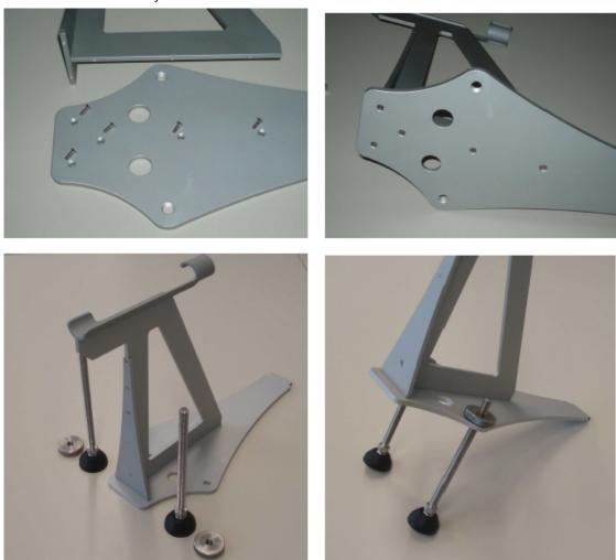
Assemble of the CryoFIT Holder Unit as shown:
