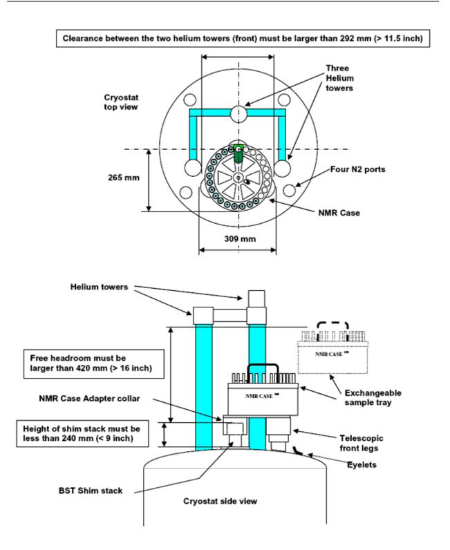
The shim stack orientation must be as shown. The two air inlets must point to the front of the cryostat. The spin rate cable connector must point to the rear. The shim cable at the bottom of the cryostat must point to the rear.
