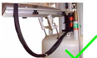
Figure 3.27. Correct installation of the cables
