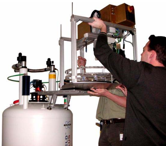
Figure 3.20. Lifting the SAMPLEJET onto the magnet
