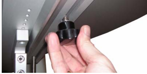
Figure 3.21. Fixing the SAMPLEJET on the platform
