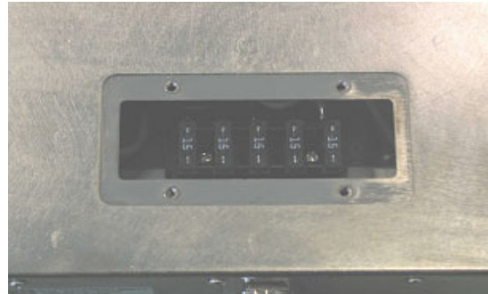
Figure 1.6. Picture of the gradient cable used with the GREAT 1/40 and GREAT 1/60 amplifiers. The filter box shown on the picture is a part of the gradient cable accessory (HZ0969)
