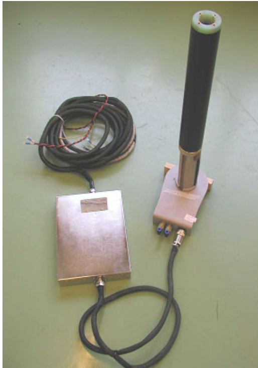
Figure 1.6. Picture of the gradient cable used with the GREAT 1/40 and GREAT 1/60 amplifiers. The filter box shown on the picture is a part of the gradient cable accessory (HZ0969)
