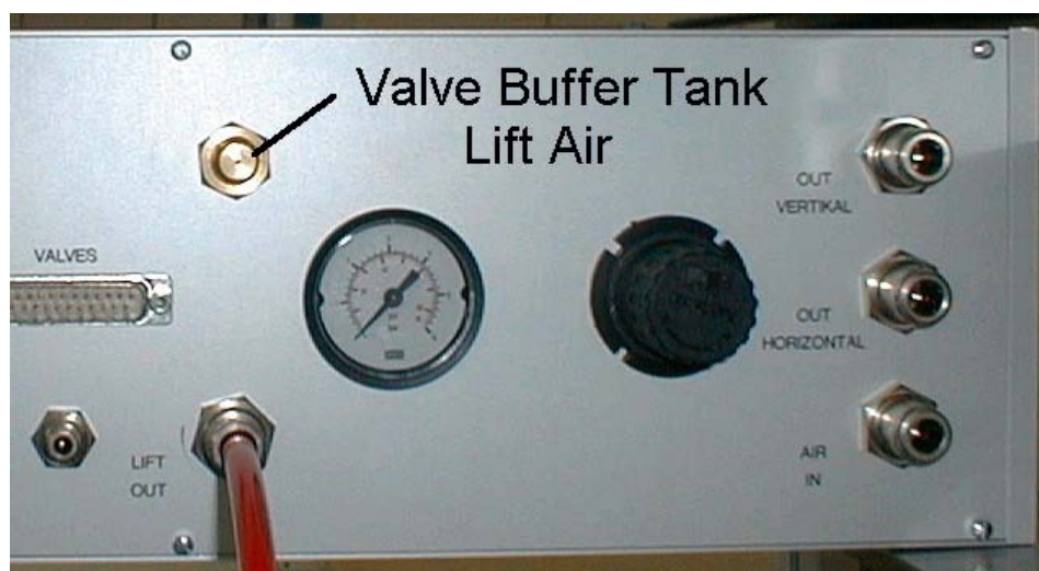
Figure 5.2. BSR Pneumatic Unit - Rear Side
