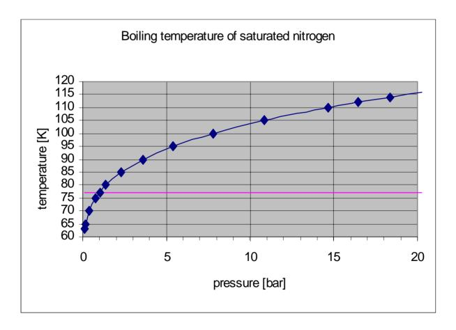
Warning:Containers for cryogenic liquids must not be closed completely<br/>as this would result in a large build up of pressure. This will<br/>present an explosion hazard and leads to large product losses!
