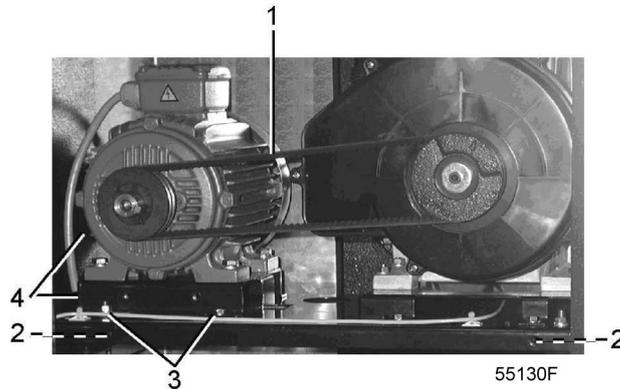
1. Loosen motor hold-down bolts (3).
