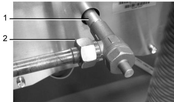
3. Remove the outlet pipe together with the check valve
