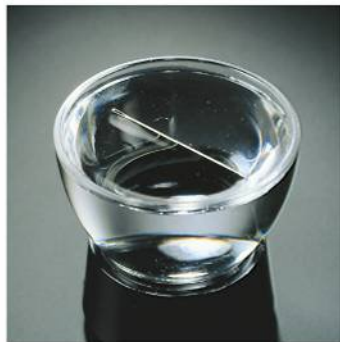
▲ FIGURE 12-10 An effect of surface tension illustrated
