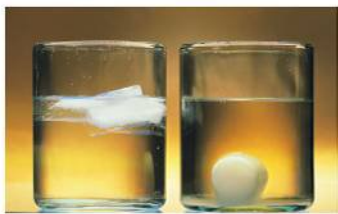
▲ FIGURE 12-8 Solid and liquid densities compared
