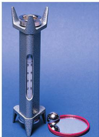
▲ FIGURE 12-15 Measuring Viscosity By measuring the velocity of a ball dropping through a liquid, a measure of the liquid viscosity can be obtained.
