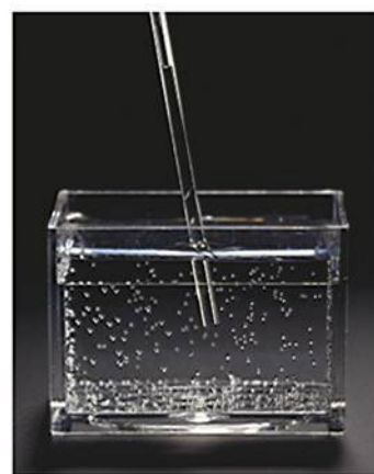
▲ FIGURE 12-14 Capillary action
